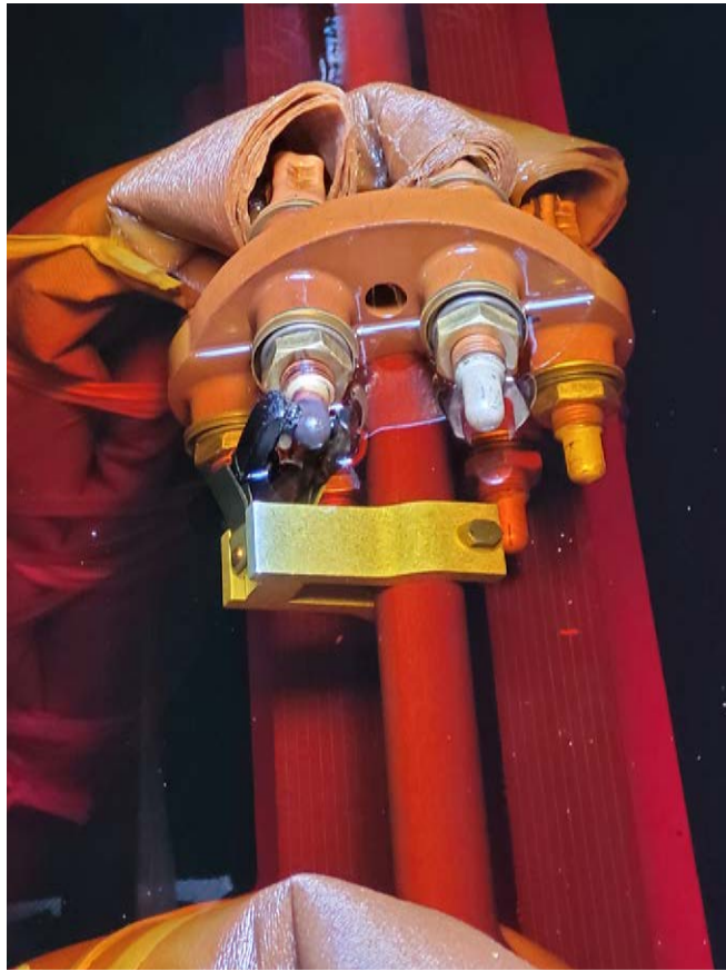
Close-up of the transformer shows carbon deposits and evidence of arcing (as seen by the dark color on the left).
